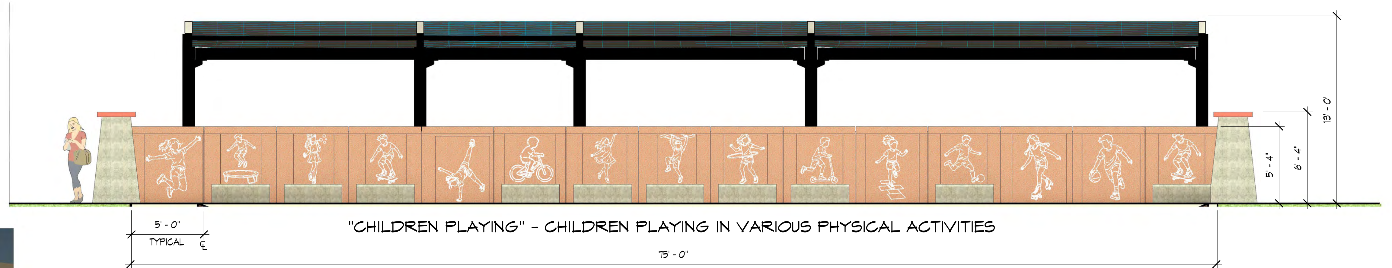
RAILING PANELS - EAST ELEVATION 1 Scale: 1/4" = 1'-0"
